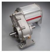
**Power Saver 3.5** 460/380 volt AC, 60/50 hz electric motor with a speed reducing gearbox that uses 95% efficient helical spur gears for power transmission on electric center pivots and lateral move systems.
